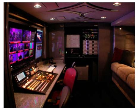
Master Control is where it all happens! All of the cameras are recorded separately on the special built server/computer system by Apple. This allows immediate access to the material for editing purposes as soon as the live show is complete.
